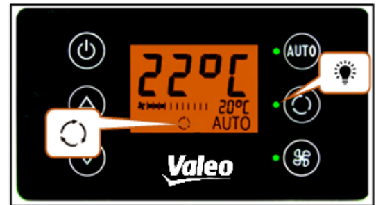
Figure 11 - SC600 recirculating air function activated
