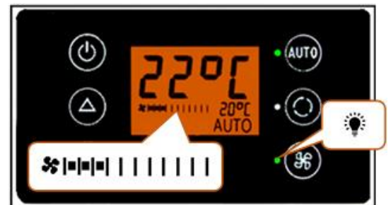
Figure 10 - SC600 setting the blower level manually
