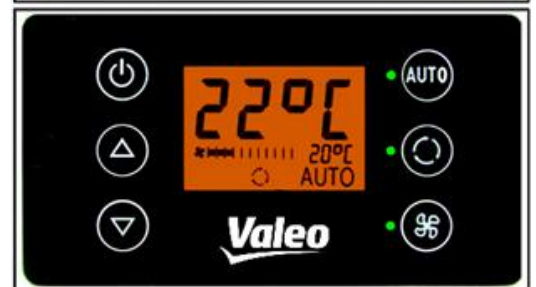
Figure 12 - SC600 setting the temperature
