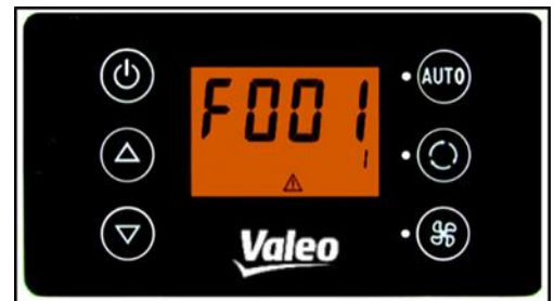
Figure 14 - SC600 Error detection mode
