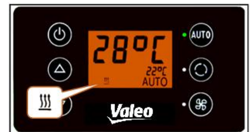
Figure 8 - SC600 Auto mode activated, Heating mode
