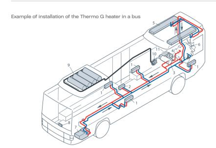
Water heating circuit - wall heaters and roof duct heating
