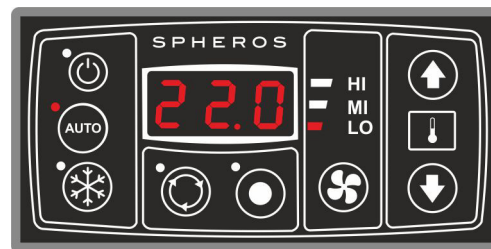
Fig. 9: SC410 The compressor of the air-conditioning unit is deactivated.
