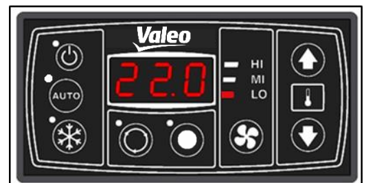
Figure 12 - SC410 blower level at low speed
