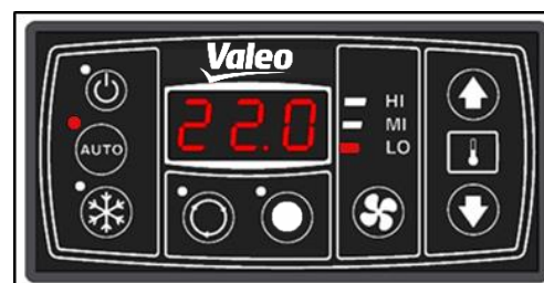
Figure 6 - SC410 air-conditioning compressor deactivated
