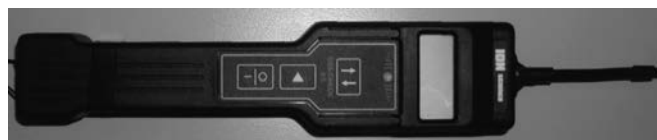
Fig. 7-8 Electronic leak detector
