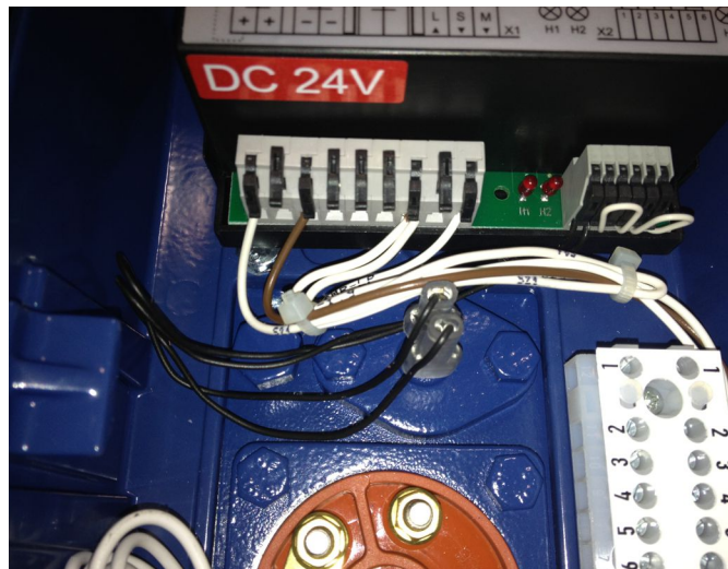
Figure 24: Junction box REVO-E without frequency converter (compact)
