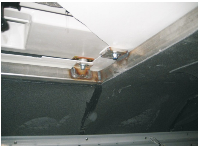
Figure 16: Fastening if using Armaflex
