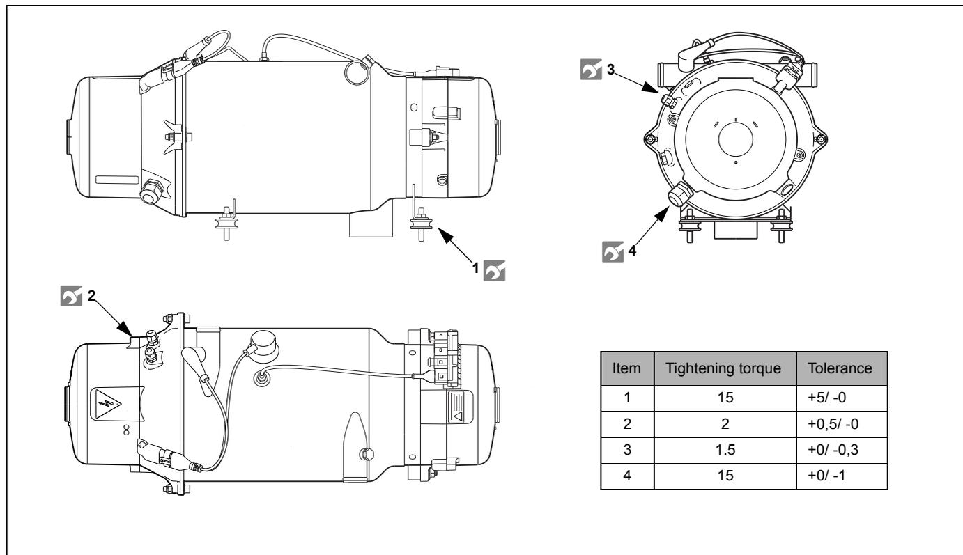
Fig. 16: Tightening torques
