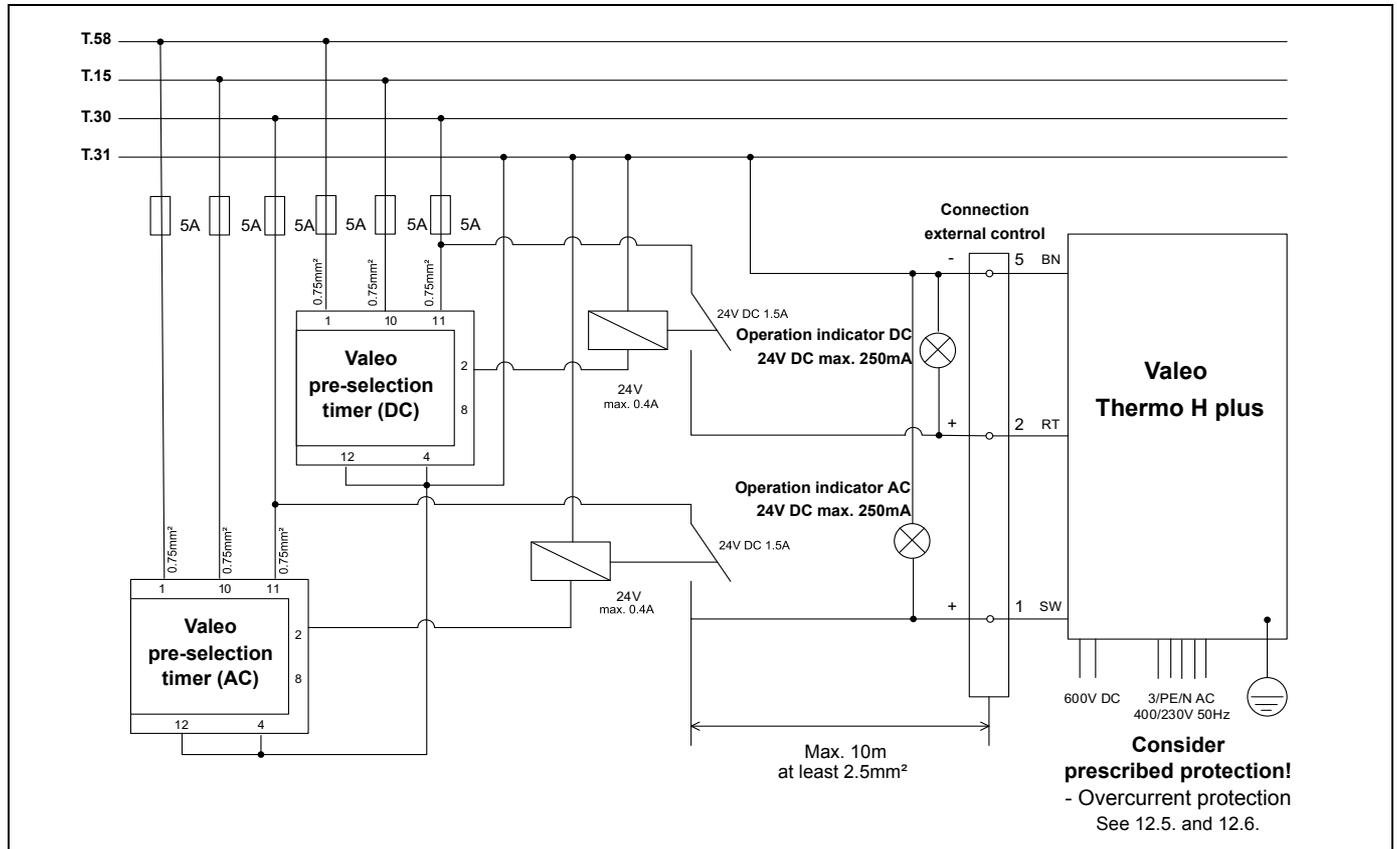
Fig. 15: Control of the electrically operated part of the heater using the pre-selection timer
