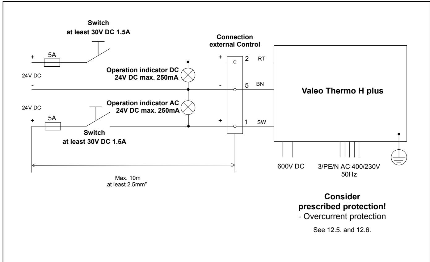
Fig. 14: Control of the electrically operated part of the heater by a switch (relay)
