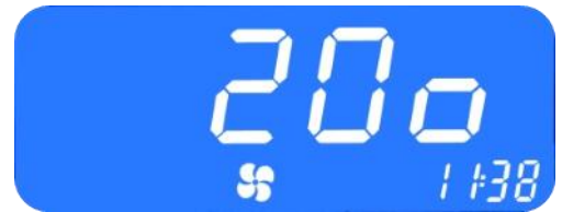
Figure 7 - SC1000 Current Blower Speed Level
