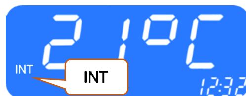
Figure 14 - SC1000 Current Room Temperature
