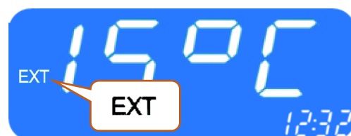
Figure 15 - SC1000 Current Exterior Temperature
