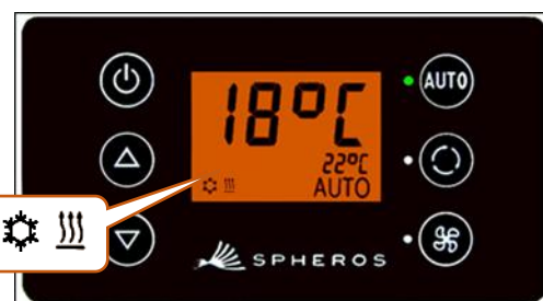
Fig. 11 - SC600 dehumidification is activated
