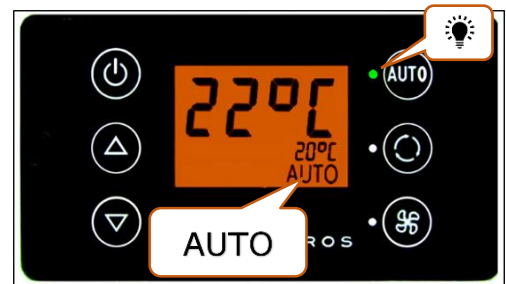
Fig. 5 - SC600 auto mode is activated
