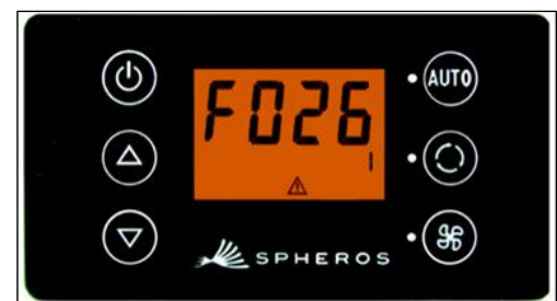
Fig. 14 - Reading out SC600 faults
