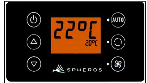
Fig. 8 - SC600 auto mode deactivated
