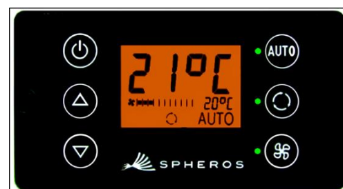
Fig. 11 - SC600 dehumidification is activated
