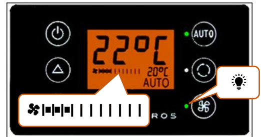
Fig. 9 - Manually adjusting SC600 blower level
