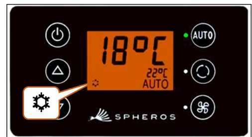
Fig. 6 - SC600 auto mode is activated, cooling mode
