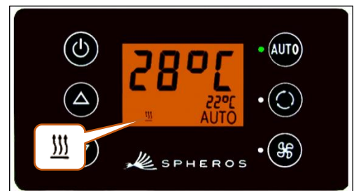
Fig. 7 - SC600 auto mode activated, heating mode
