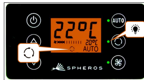
Fig. 10 - SC600 Circulation function activated
