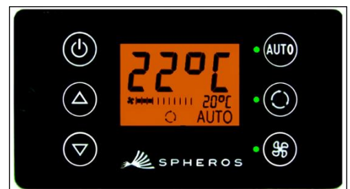
Fig. 15 - Standard SC600 operating display
