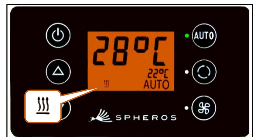
Figure 8 - SC600 Auto mode activated, Heating mode
