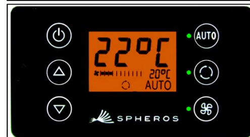
Figure 12 - SC600 setting the temperature
