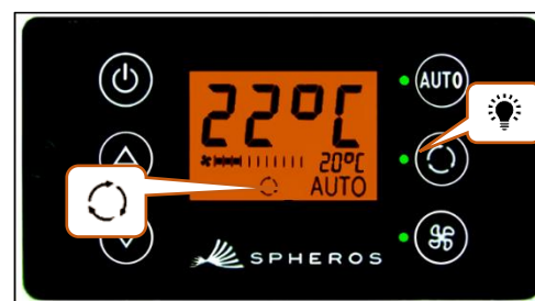
Figure 10 - SC600 recirculating air function activated
