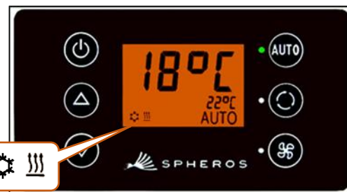
Figure 11 - SC600 dehumidify activated
