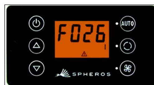
Fig. 14 - Reading out SC600 faults
