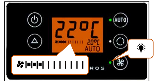
Figure 8 - SC600 setting the blower level manually
