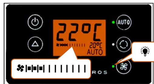
Figure 10 - SC600 setting the blower level manually
