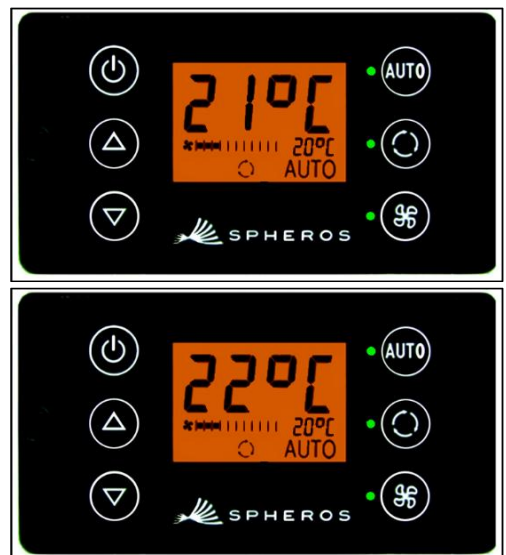
Figure 12 - SC600 setting the temperature
