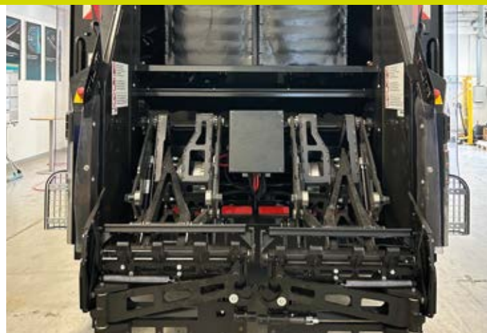
The vehicle cleans dirty rubbish bins with hot water as they are being emptied.
