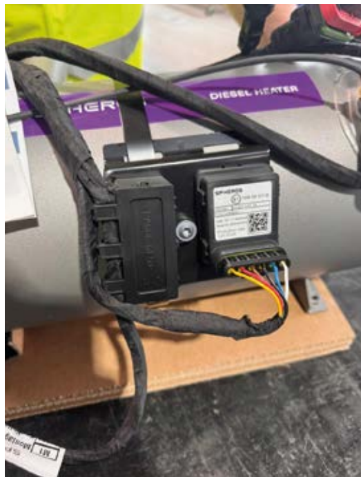
Heater with a visible gateway module.
