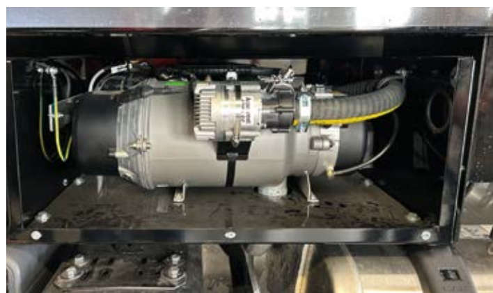
At the heart of the Thermo H plus is its hybrid heating system, which can run on both electricity and diesel.
