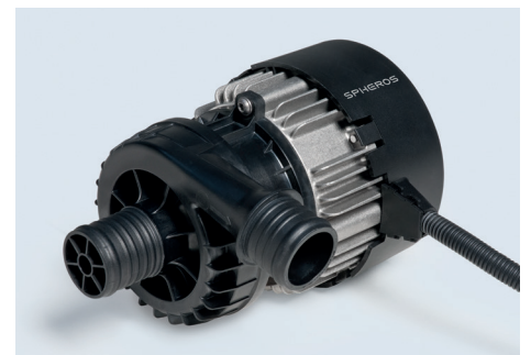
Powerful SPump specially developed for use in electromobility and battery cooling (high counter-pressure), long life (magnetically coupled, brushless), CAN interface.
