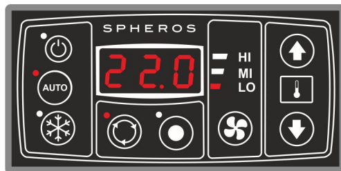
Fig. 15: SC410 Circulating air mode is active
