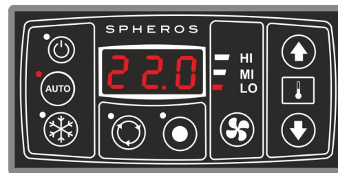
Fig. 9: SC410 The compressor of the air-conditioning unit is deactivated.
